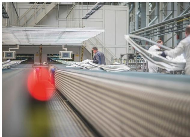
At the Volkswagen Emden factory, doors, hoods, trunk lids, or entire side sections of the current Passat B8 are formed on two parallel-running press lines.
