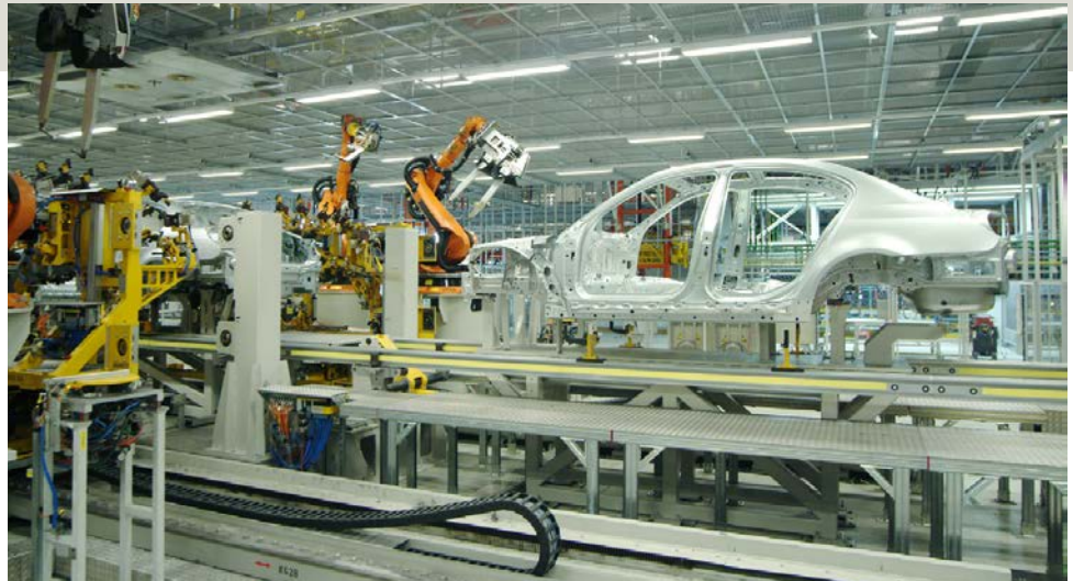
KUKA framing in body shop.
