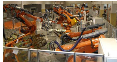
An automotive body-in-white production line tested by KUKA Brazil prior to shipment.
