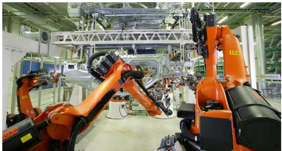
An automotive body-in-white production line delivered by KUKA Brazil.
