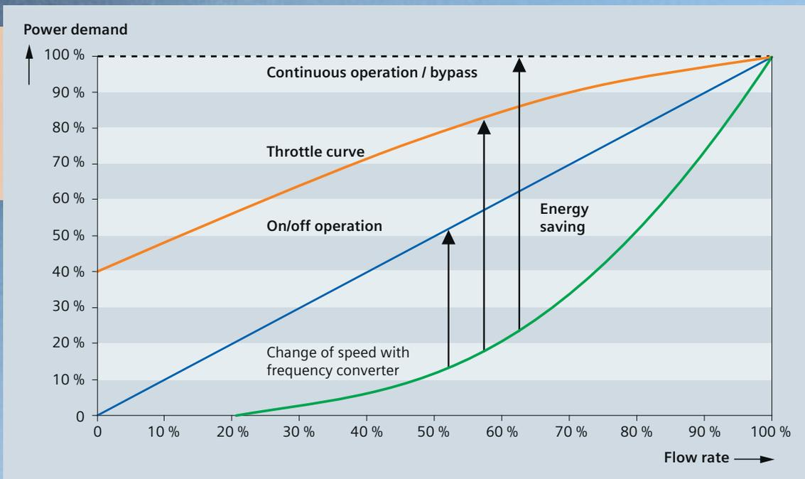
Savings potential of throttle, 2-point control, and pump cascades depending on the production rate
