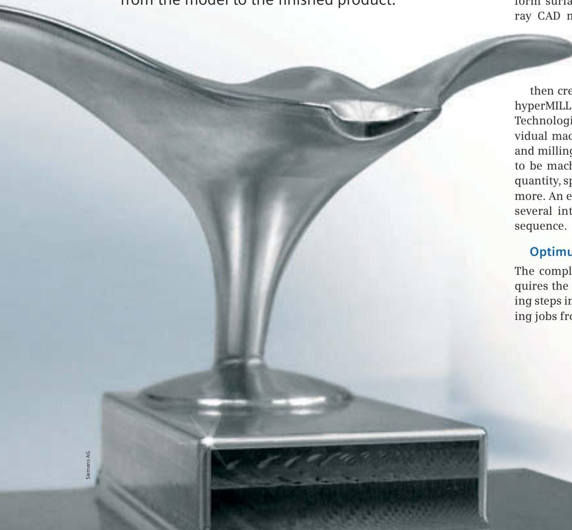
both fixed and simultaneously moving rotary axes. When defining the jobs, tolerances for calculation accuracy are specified. These are usually 0.1 millimeters for rough machining and between 0.005 and 0.001 millimeters for smoothing operations. These tolerances must be subsequently factored in during the production phase.
