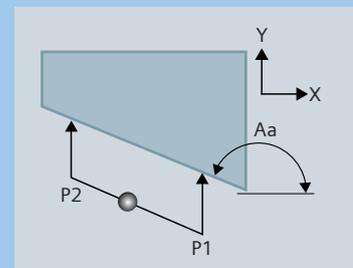
with the EasyProbe measuring program. The measuring probe is moved to the appropriate start position in JOG or MDA mode, without needing to create an NC parts program. In MDA mode, the operator calls up the corresponding measuring cycles directly. EasyProbe allows the operator to program standard measuring cycles quickly and easily – without
