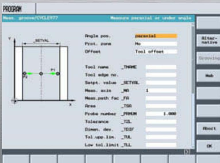
Automatic process measuring cycle: groove measurement with tool correction
