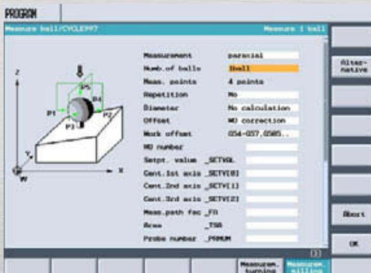
Automatic process measuring cycle: sphere measurement with zero point correction
