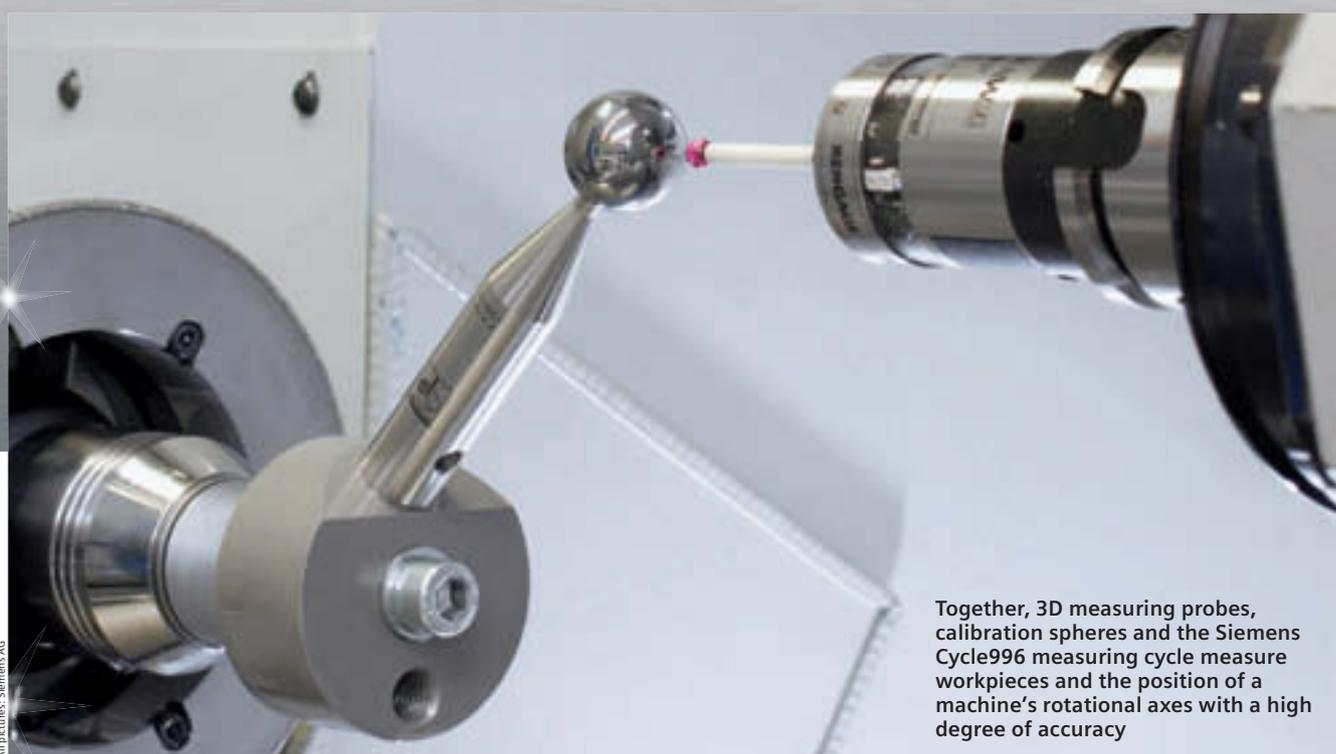
Together, 3D measuring probes, calibration spheres and the Siemens Cycle996 measuring cycle measure workpieces and the position of a machine's rotational axes with a high degree of accuracy
