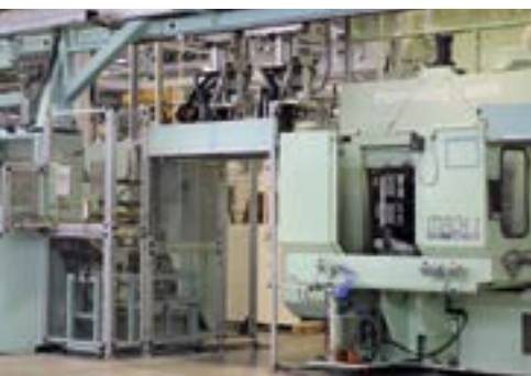
Loader and grinding machine – camshaft line
