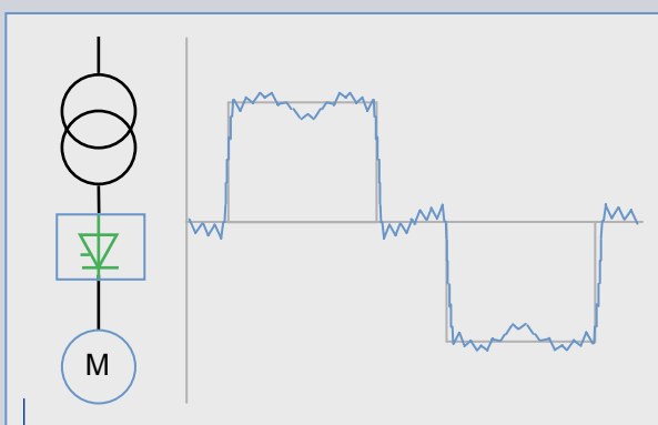
The DC blocks of the power converter consist of the fundamental component and the overlaid harmonic components
