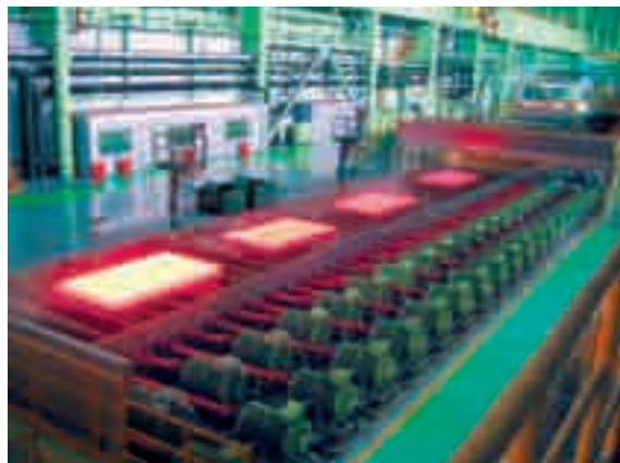
Automated thermo-mechanical rolling in "batch mode" increases mill utilization
