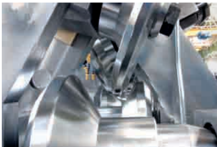
View of a typical roll configuration of an FCF line
