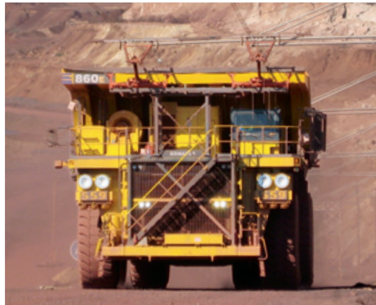
The new Siemens drive system will power the recently announced Komatsu 860E-1K truck
