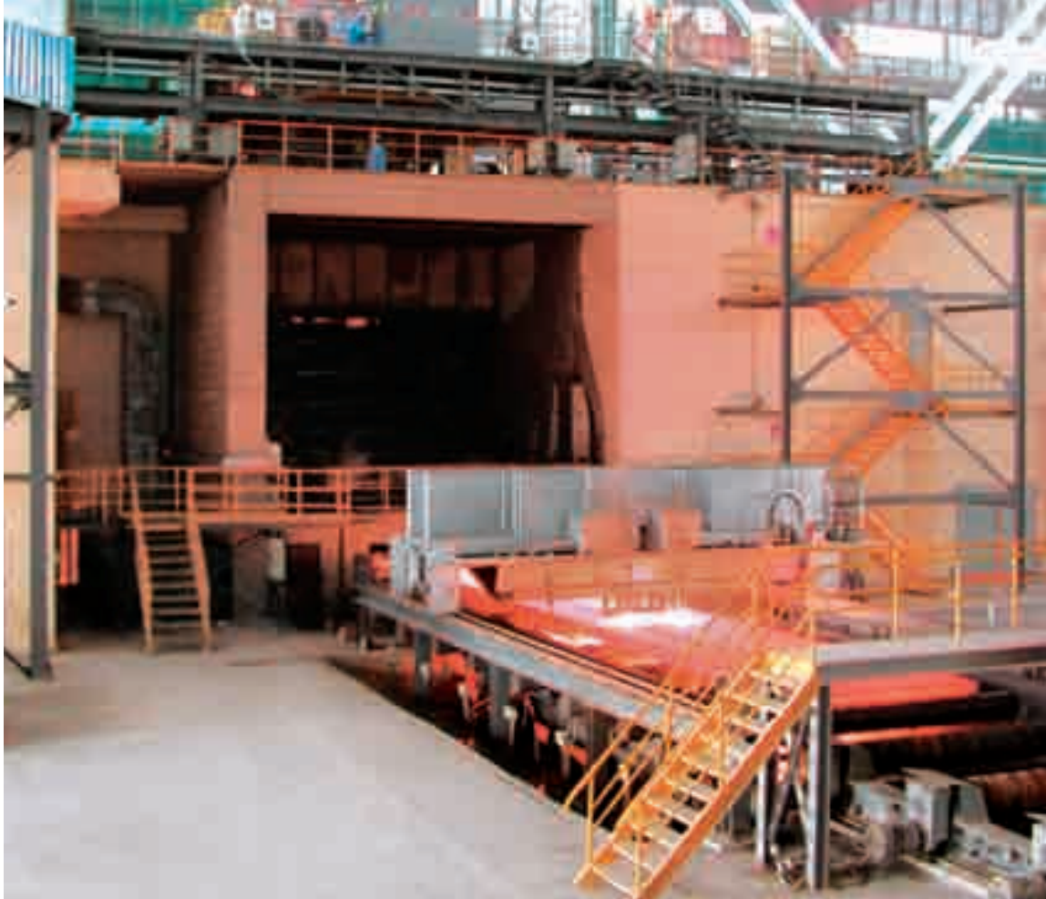
Single-strand, ultra-wide, medium-thick-slab caster, Nanjing Iron & Steel Co., China
