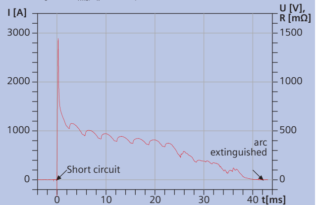
Switch-off diagram U_0: 925\text{ V}_{\text{rms}}, I_k: 150\text{ kA}, dI/dt: 12\text{ kA/ms}
